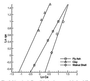
Fig. 5: Linearized Freunlich isotherm model for MB adsorption on various adsorbents
